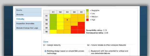
The criticality of the asset equipment can be assessed with customisable susceptibility /consequence of failure ratings, criticality matrix size and threshold values.
