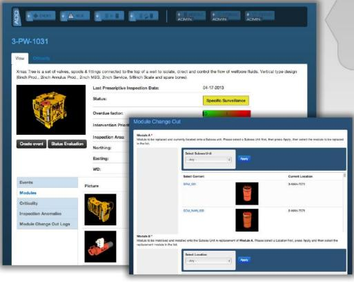
Modules are attached to Subsea Units or storage locations (yards, workshops, vessels...). All movements and change out operations can be logged in the database. Associated logs are then auomatically attached to the involved units, modules, and storage locations.
