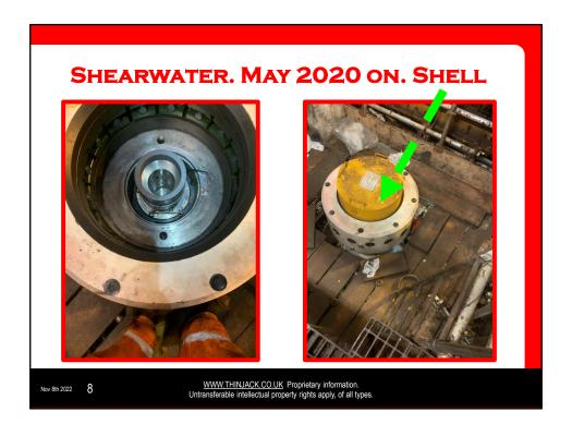
This is one of three guards for protecting flanges at the tree cap, base of XMT and the base of a spool.
