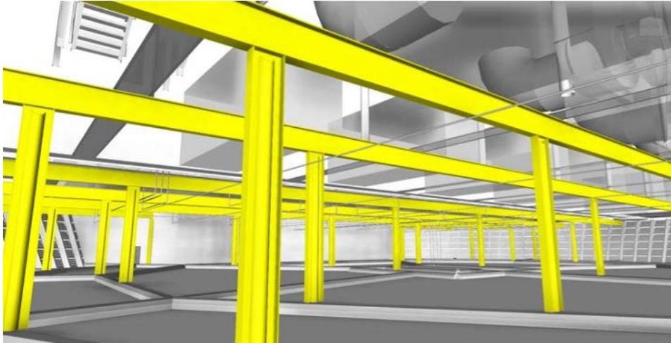
Figure 15.4-15-26: Example Pillar/stooling arrangement
