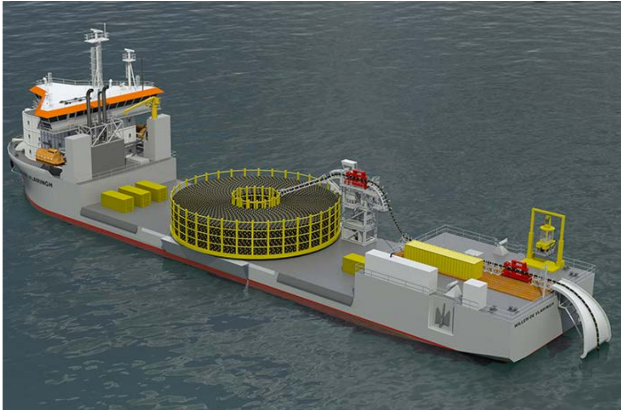
Figure 17-10: Cable Lay Vessel Operations Example (Reference /77/)
